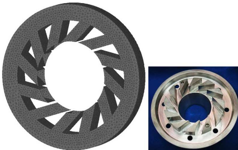
Fig. 8. Detail of the mesh at the swirler of the Turbomeca injector.
