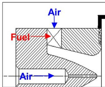
Fig. 1. Turbomeca low emissions injector.
