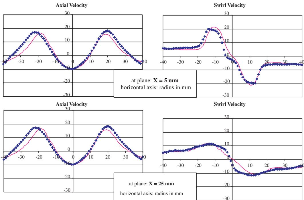
Fig. 11. Cold flow velocity comparisons at 5 and 25 mm between LES (lines) and measurements (dots).
