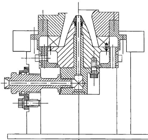
Fig. 2. Adaptation of the TM's single swirler injector to the DLR's gas supply holding the burner on their Stuttgart test rig.
