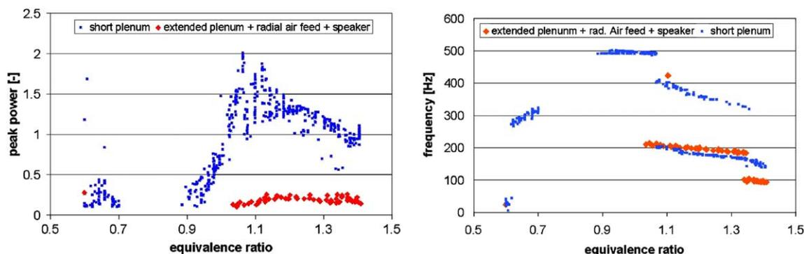
Fig. 4. Amplitude (left) and frequency (right) of the dominant self-excited oscillation as a function of equivalence ratio.
