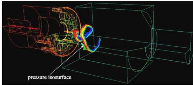
Fig. 10. Visualisation of a “precessing vortex” by pressure iso-surfaces.
