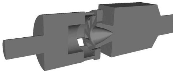
Fig. 7. Cross cut of calculation domain showing radial swirler feed and laboratory combustor.
