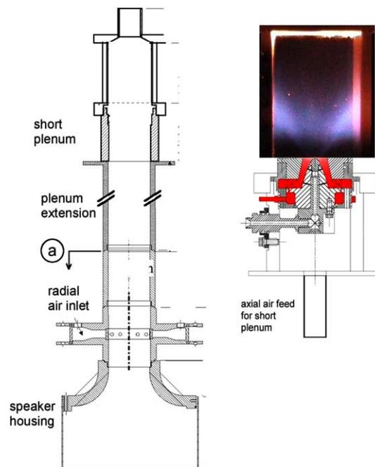
Fig. 3. Burner and Plenum design for different configurations. Section below “a” is removed for measurements shown with square symbols in Fig. 4 Top right: Visible flame shape.
