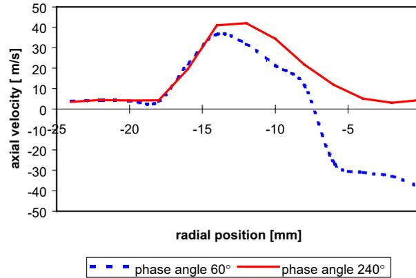
Fig. 5. Phase-coupled axial velocity measurements.
