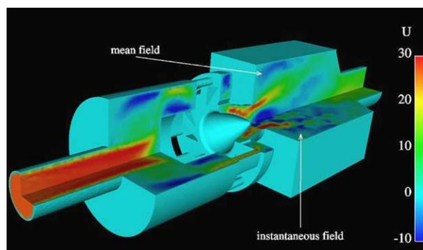
Fig. 9. Mean and instantaneous flow field of the axial velocity component U.
