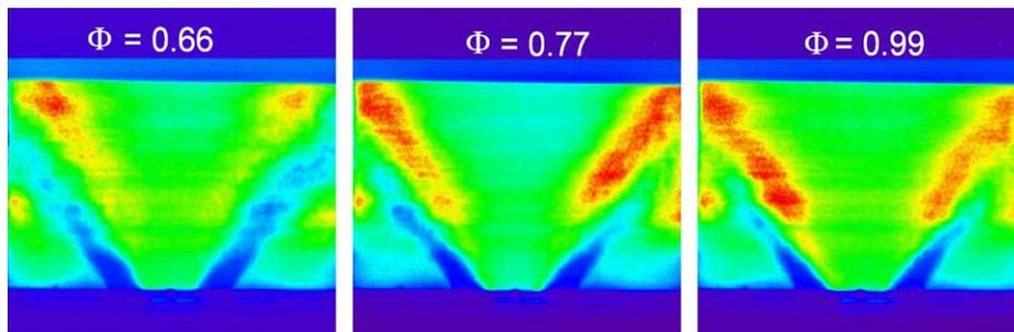
Fig. 6. Time-averaged OH distributions in the 35 kW flame at different equivalence ratios.
