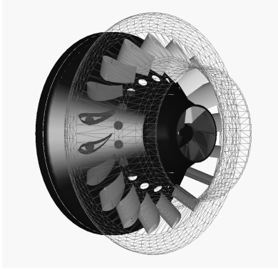
FIGURE 4. Burner: the vanes of the diagonal swirler are not computed
